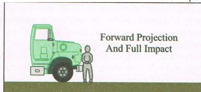
Exhibit 32. If a standing adult pedestrian is struck by a fairly flat front vehicle such as a truck, van, or bus, he will be accelerated to the same velocity as the vehicle.
