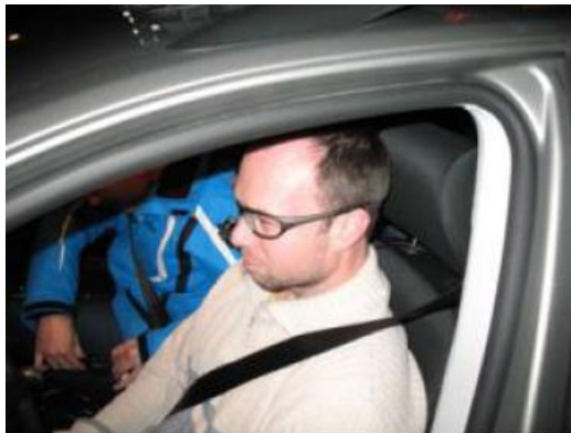
Fig. 4: Driver wearing frames shaped as spectacles, with two cameras for measuring his direction of vision
