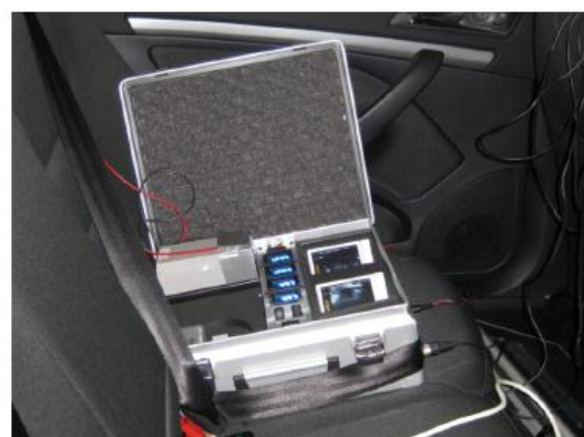
Fig. 7: Data logger HOLUX M-241, which, among other things, synchronises the instrument recordings
