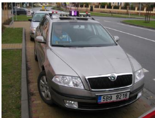
Fig. 5: Vehicle Škoda (F_H7) with fitted IR floodlight to ensure good quality recording of the IR camera
