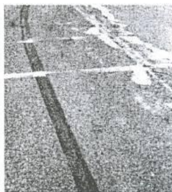
Exhibit 3. A typical skidmark on bituminous pavement is clearly visible.
