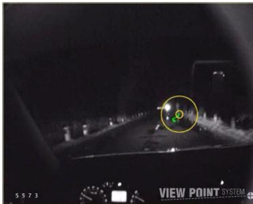
Fig. 8: Example of determining the driver's angle of vision using the viewpointsystem® method – low beam. Data merged by the evaluation software
