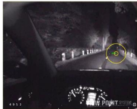
Fig. 9: Example of determining the driver's angle of vision using the viewpointsystem® method – high beam.
