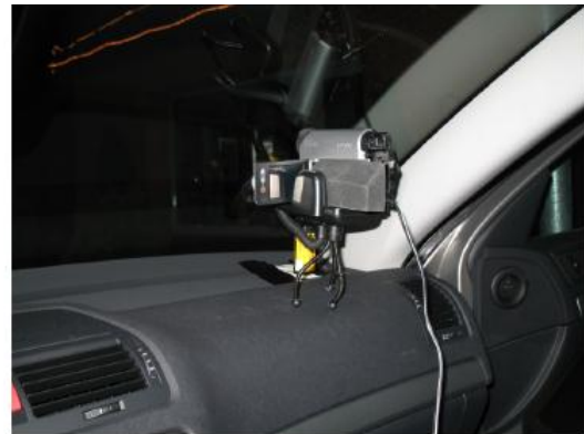
Fig. 6: Fixed camera for determining the moment the vehicle passes the actor-pedestrian
